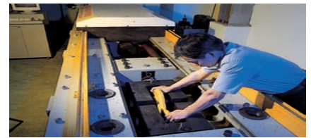
Tensile Test, Capacity 300 tonnes
